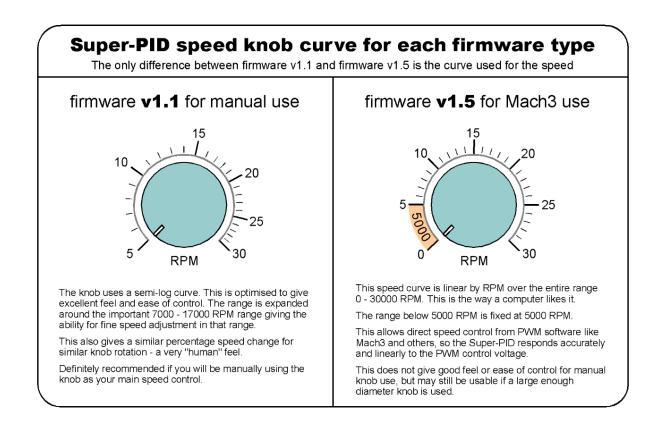
These modes set the speed curve used for the speed control system. One curve is best suited for manual use (with a knob) the other curve is optimised for computerised speed control using Mach3 or EMC or other PC CNC software.
