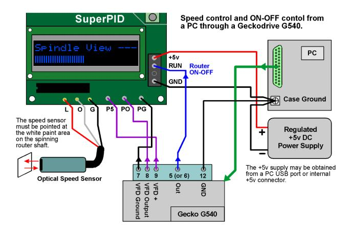
This is a common and popular setup where the G540 produces the 0v to 5v speed control voltage and also produces the router ON - OFF control signal.
