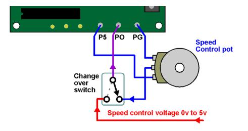
The diagram shows how to switch between a speed control voltage and the speed pot.
