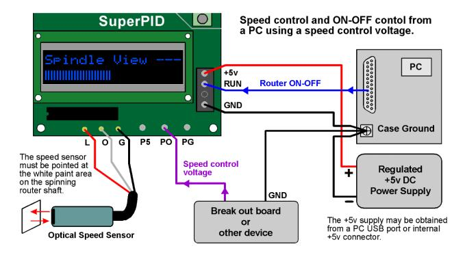
This shows connection to a PC parallel port to provide router ON - OFF control, and to a separate device that produces the 0v to 5v speed control voltage, sometimes called a "VFD control voltage". Below shows a popular alternative connection where both signals are produced by the break out board or other device.
