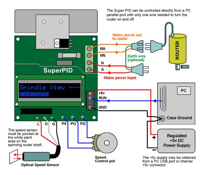
This is a popular method of connecting the Super-PID. The PC can turn the router on and off, but the speed control is still adjusted by hand.
