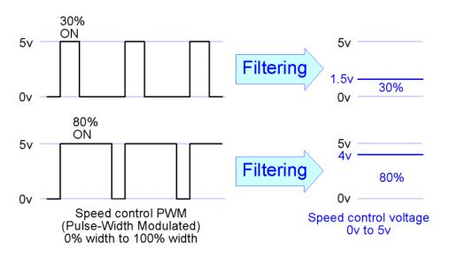
If you have a PWM signal from a CMOS logic level pin (like most breakout boards, Smoothstepper etc) it can be filtered with a simple resistor and capacitor, and the filtered signal applied to the Super-PID "PO" terminal instead of the signal from the pot.
