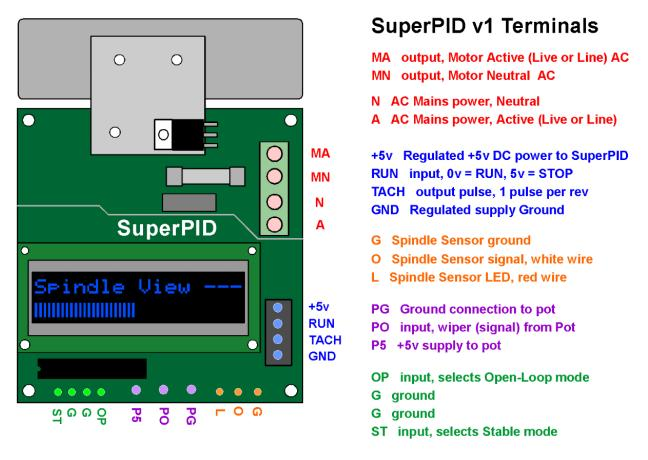
Notes; If using Mach3 speed control from a PC, connect a filtered speed control voltage (ranging from 0v to 5v DC) into the **PO** terminal and disconnect the pot.
