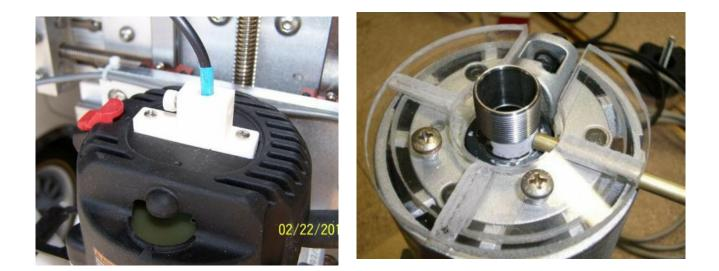
Here are some spindle RPM sensor mountings, at the top or bottom of the router.
