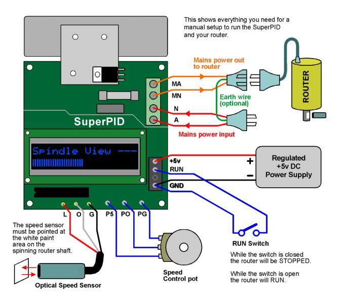
This is the minimum setup to operate the Super-PID manually.
