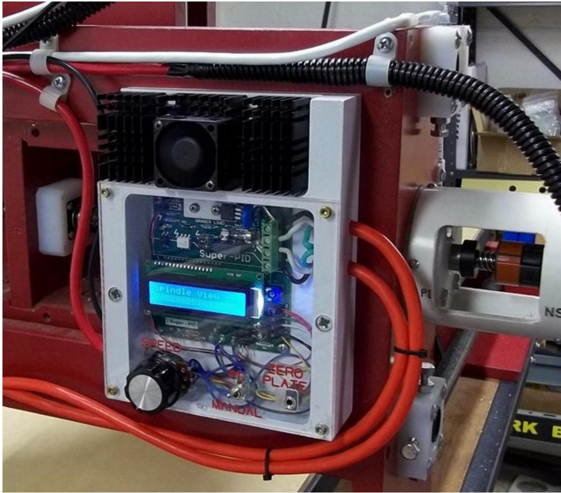
Above shows a neat custom shaped enclosure with external heatsink.
